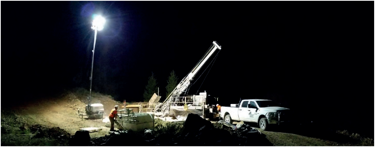
Night shift diamond drilling
